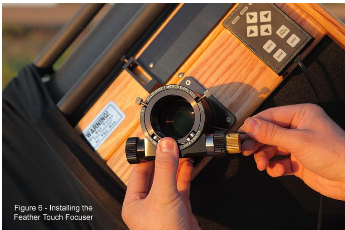
Figure 5 - Installing the Feather Touch focuser
